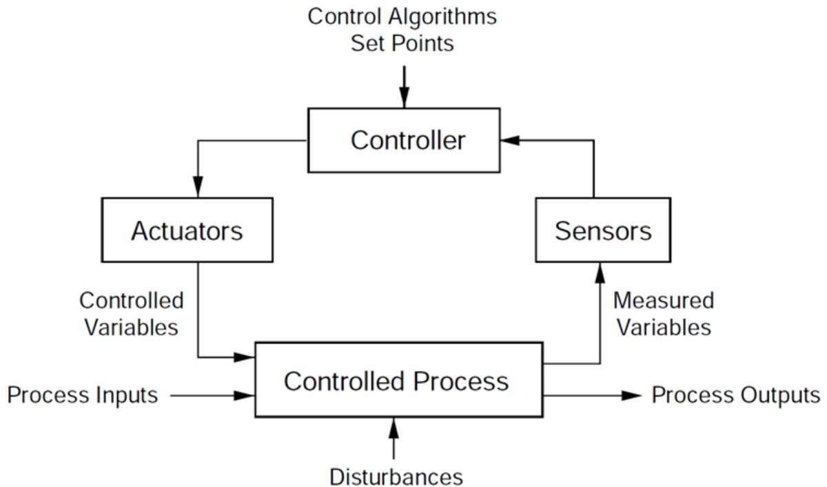
**Figure 1 A standard control diagram (Leveson, 2011, pp. 66)**
