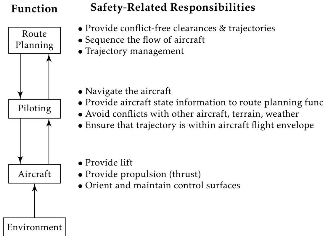
**Figure 16: High Level Control Structure & Responsibilities**
