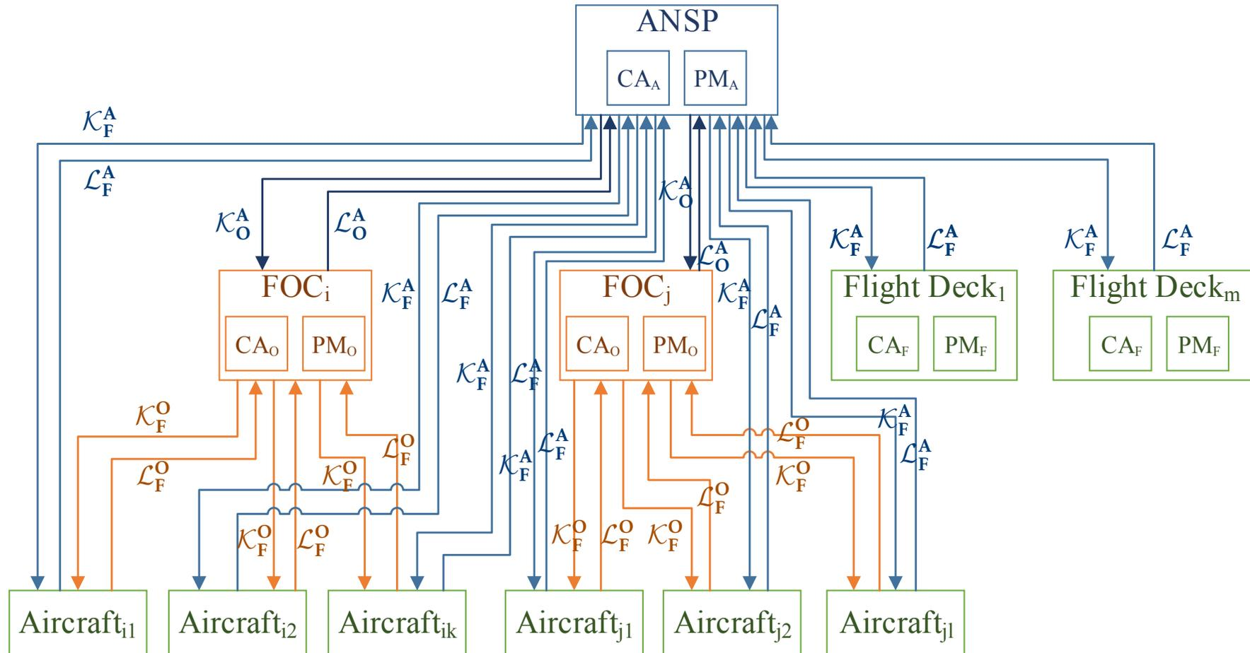
Figure 27: Nominal TBO Control Model—Trajectory Negotiation
