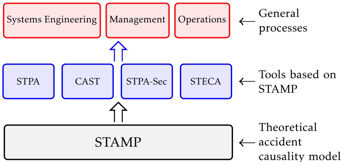
**Figure 7: Techniques based on STAMP Accident Causality Model**
