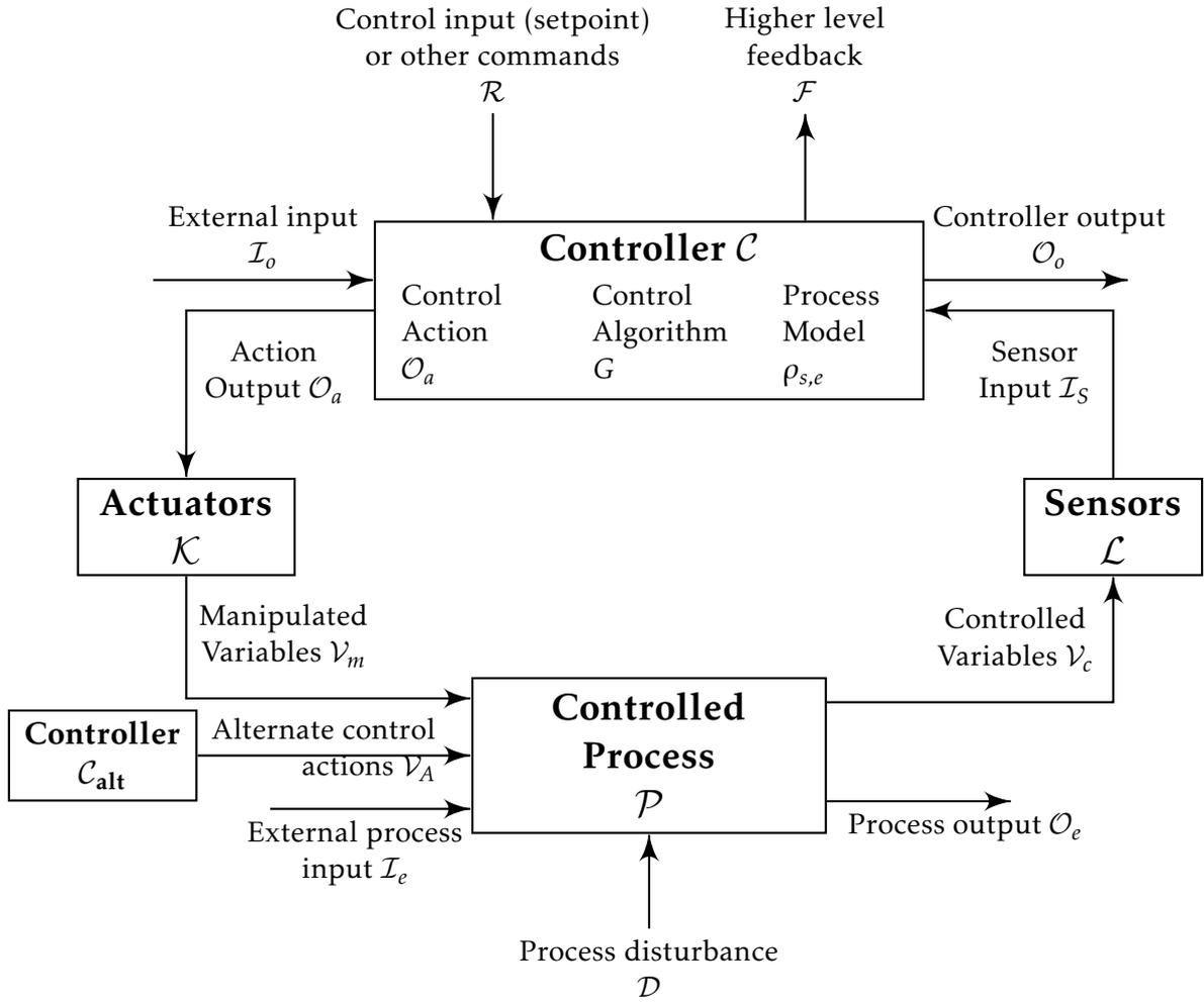
**Figure 13: Generic Process Control Loop**
