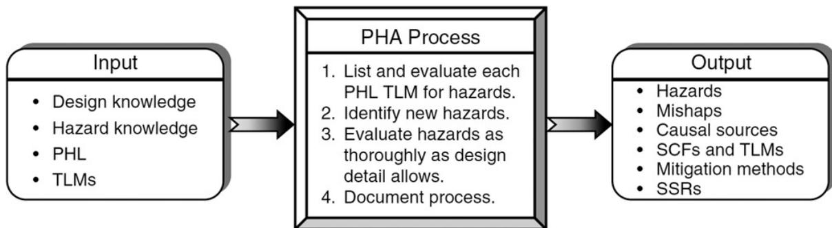
**Figure 3: PHA Inputs, Process, and Outputs [Ericson, 2005]**
