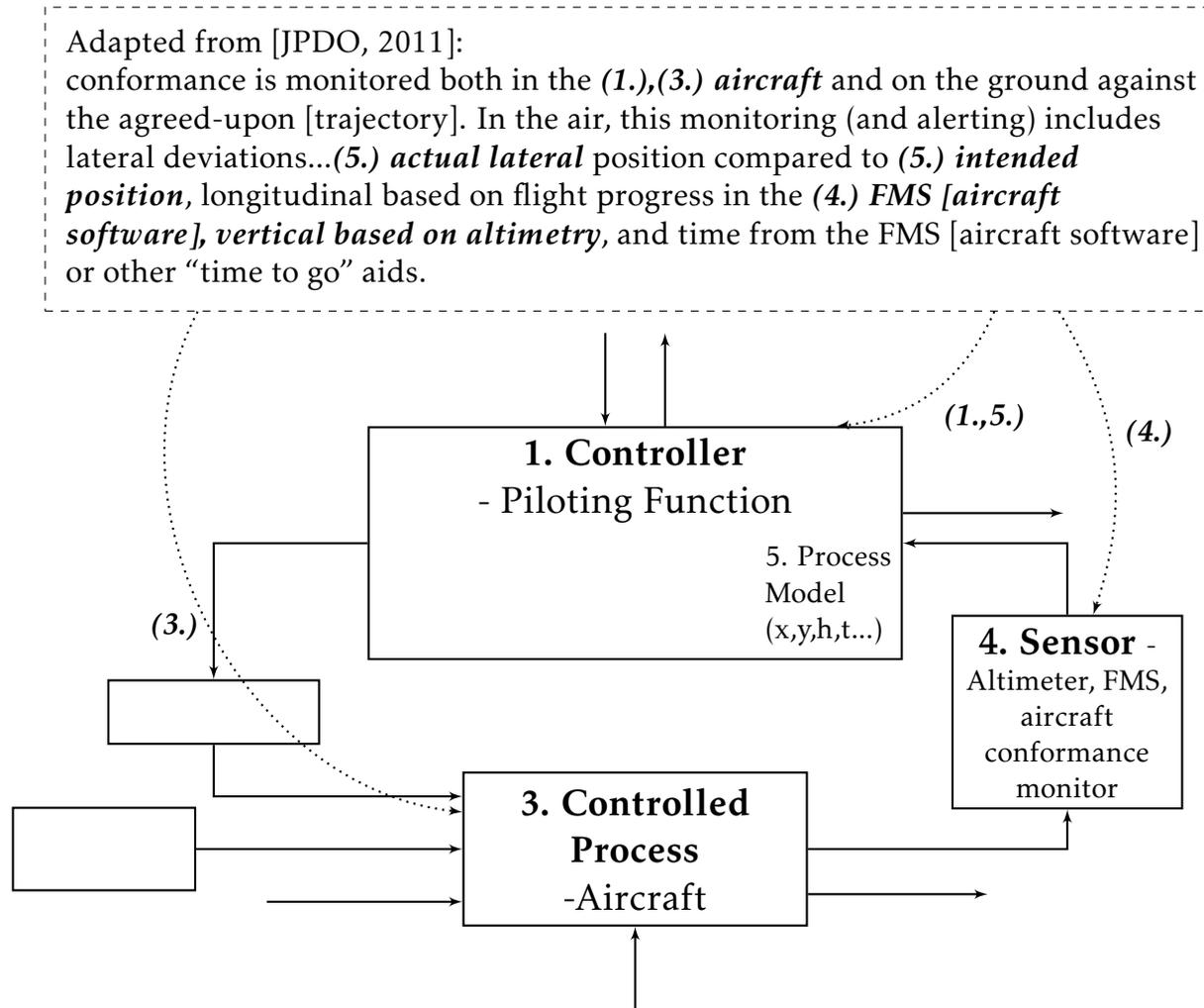
Figure 18: Graphical Control Model of Airborne Conformance Monitor
