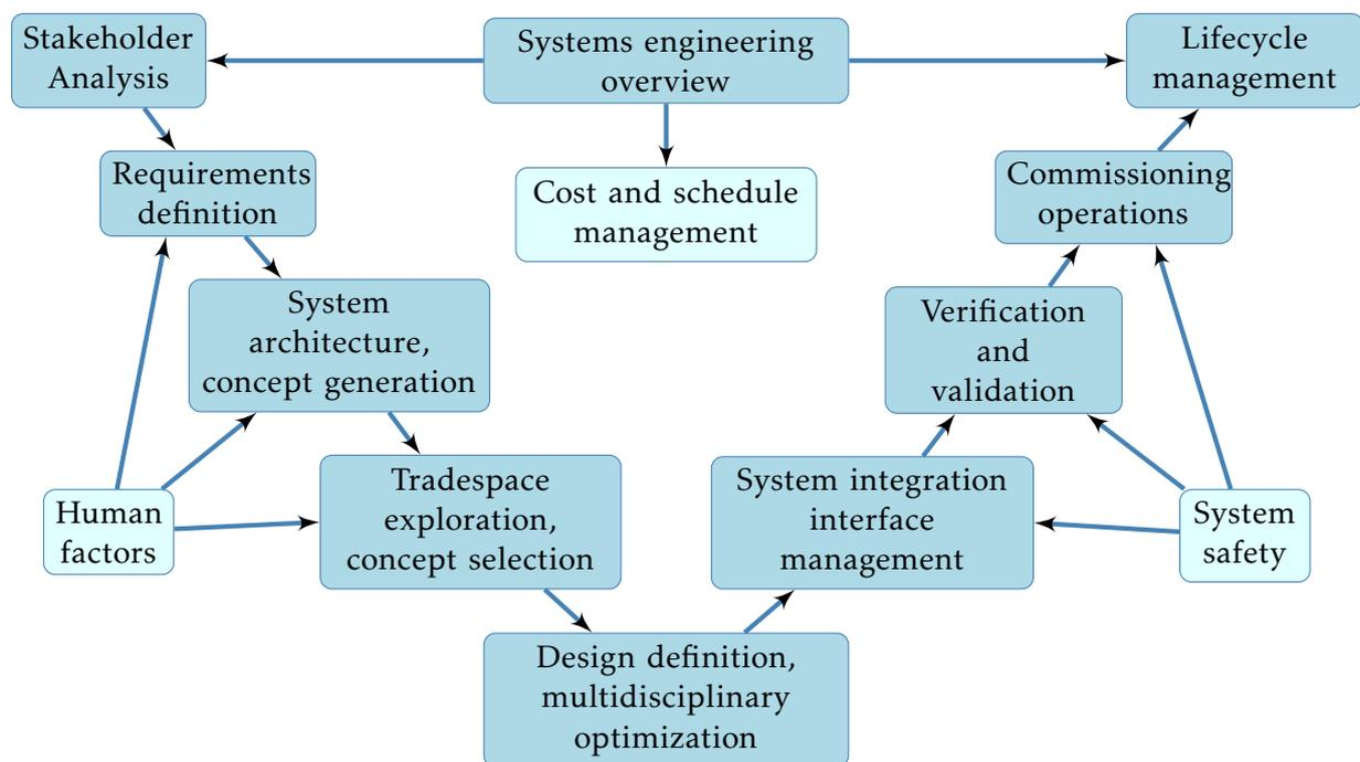
Figure 2: System Engineering Vee Model [de Weck, 2009]
