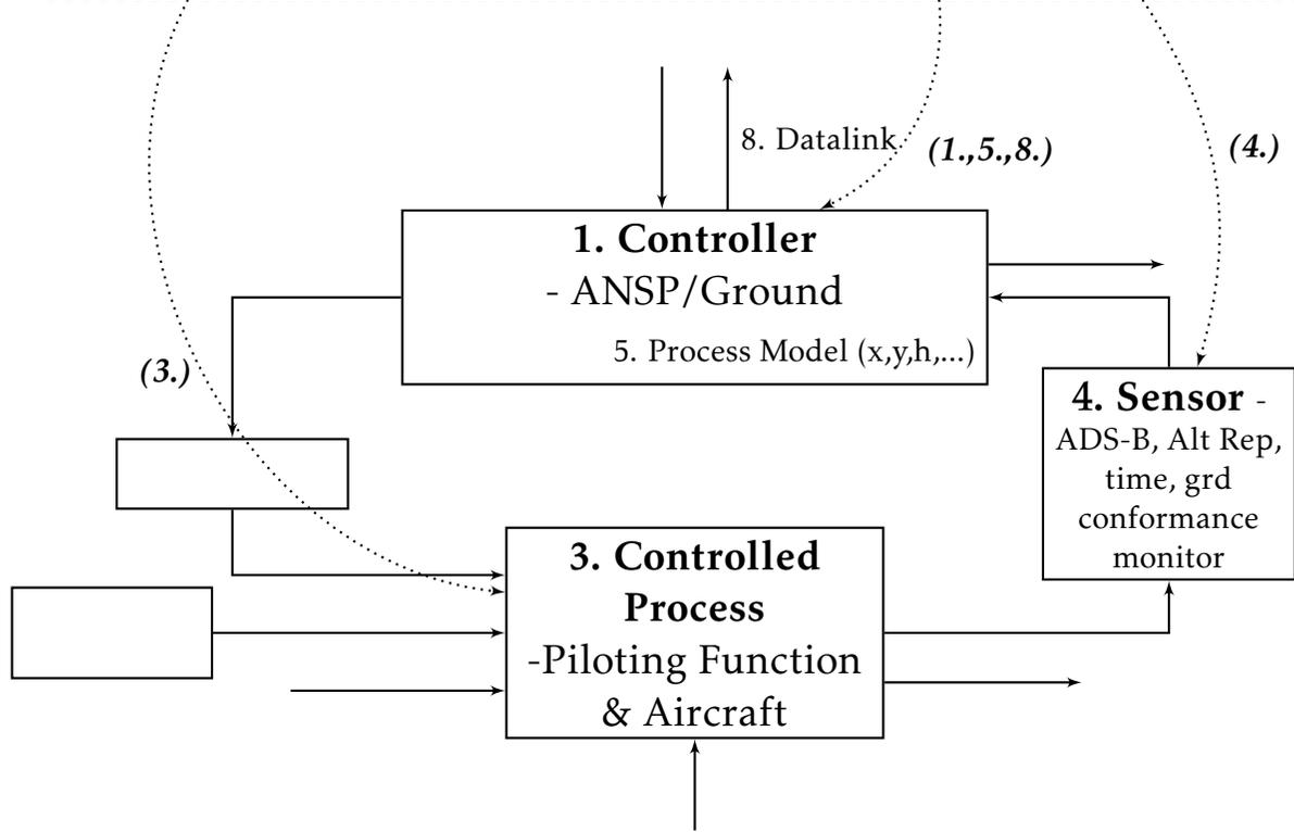
Figure 19: Graphical Control Model of Ground Conformance Monitor
