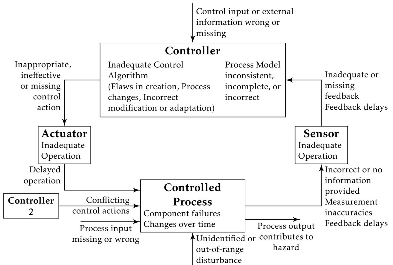
Figure 10: STPA Control Loop with Causal Factors
