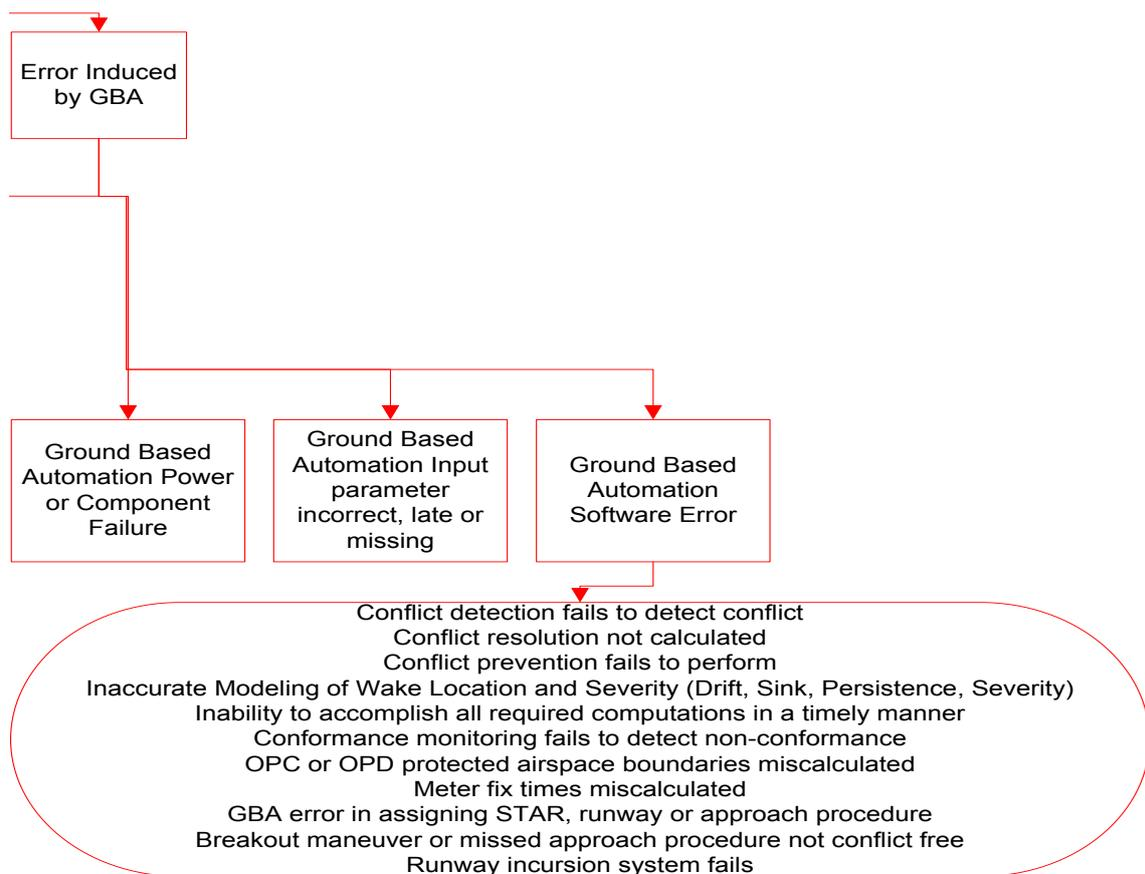
**Figure 31: Software in Fault Tree Analysis [JPDO, 2012]**
