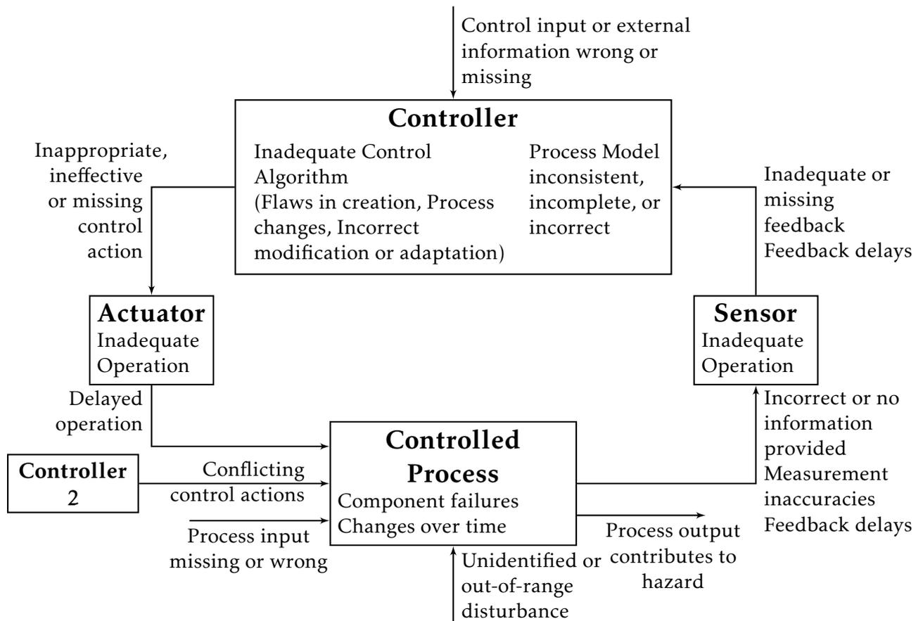
**Figure 6: STPA Control Loop with Causal Factors**
